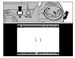
To select the Exposure Compensation setting, hold down the "≥" button and turn the Command dial. The symbol indicating the compensation direction ("-" or "+") turns yellow. The "≥" symbol also turns yellow while exposure compensation is being set and then turns blue after setting is completed.
